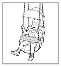
Rotate the tray back into place and push down on it to "snap" it into place. Pull up on the tray to be sure it is securely latched.
